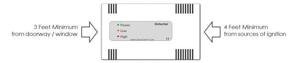
Take in to account the design of the air flow within the space. Positioning CO detectors near draft will greatly diminish their reliability. Multiple detectors may be required to adequately protect the space.
