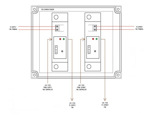
Please note: The live feed taken from the fan speed controller is to be passed through the hole in the centre of the CS switch and wrapped around the coil to increase sensitivity of the current sensor.
