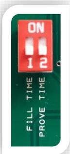
**FILL TIME** is the amount of time the gas valve is open to fill the gas line.
