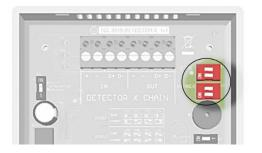
When wiring multiple detectors to the GDP-X range it is important to identify each detector and in which monitoring zone the detector is located - for the GDP-X system to receive and display accurate data.
