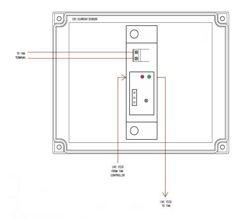
Please note: The live feed taken from the fan speed controller is to be passed through the hole in the centre of the CS switch and wrapped around the coil to increase sensitivity of the current sensor.
