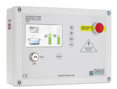
The Merlin 3000S is an energy saving system designed specifically for commercial kitchens. The system acts as an interlock between the ventilation and the gas solenoid valve, while also varying the speed of the ventilation via 0-10VDC output.
