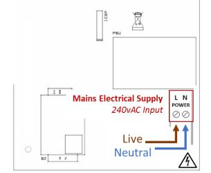
When mains supply is connected, the device will power up for 60 seconds and CO2 levels will then be displayed.
