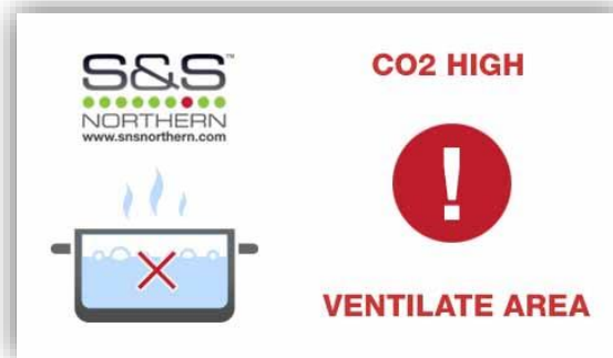
Fig.3.4 CO 2 detected fault display screen.
