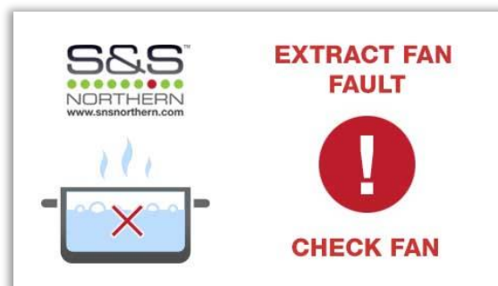
Fig.3.9 Extract fan fault display screen.
