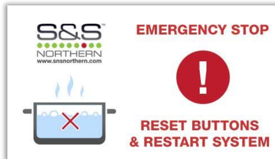
Fig.3.2 Emergency Stop fault display screen.
