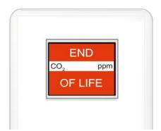
The gas monitoring elements are expected to last for 10 years from initial installation and power up depending on environmental factors.
