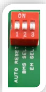
The Merlin 1000V+ can be integrated with a BMS to make or break a circuit on gas on/gas off, (valve open or valve closed).
