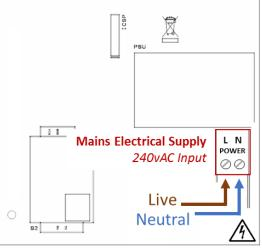
When mains supply is connected, the device will power up for 60 seconds and CO2 levels will then be displayed.
