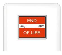
The gas monitoring elements are expected to last for 10 years from initial installation and power up depending on environmental factors.
