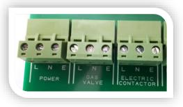
An electrical output can be supplied to an electrical contractor. This should be fused at 3A and connected to the terminals marked [ELECTRIC CONTACTOR LNE].
