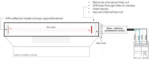
Sensor wired to Merlin 3000S circuit board
