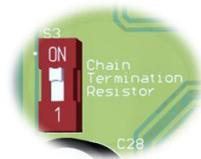
In some cases, it is also required to turn on the resistor of the first device also, e.g. If a split chain is used, terminate the last detector in each chain. If a single chain is used, terminate the first (panel) and last (detector) device.
