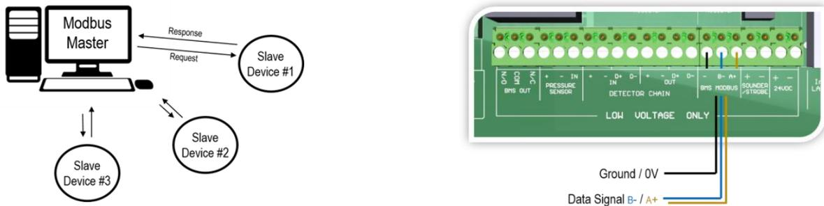
For MODBUS communications, a shielded and twisted cable is used.
