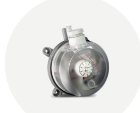
An air pressure differential switch is a mechanical switch fitted in ductwork which can be used to monitor and check airflow rates. These switches are adjustable and have a range from 20-300PA. They also come with a 1m duct kit to be fitted into the ductwork to detect the airflow.
