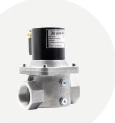
Our gas solenoid valves are 230V powered, normally closed, auto-reset and will most commonly be powered from our Merlin gas safety systems. In the event of an emergency, the Merlin gas safety system will take power away from the gas solenoid valve causing it to slam shut, and when power is re-instated this will then allow gas to flow through the
