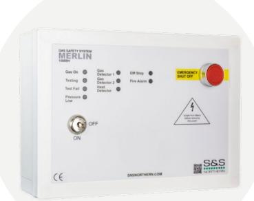
The Merlin 1000BH is a gas pressure proving and gas detection panel for use in plant rooms and boiler houses. This panel is to be used to carry out a gas proving test on the pipe work in order to highlight if there is a gas appliance open or a gas leak. The Merlin 1000BH is designed to give the user full control over the incoming gas supply with the lockable keyswitch operation.
