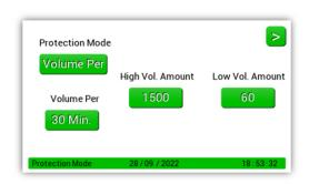
In this mode the system will allow a set amount (volume) of water through the pulse meter during a defined period. By combining these values, you increase/decrease the sensitivity of the systems measurement of flow volume. To edit the flow volume, press the button under the high or low volume value you wish to adjust. Use the arrows to adjust values, press enter to save and return to the screen shown.
