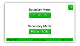
Pulse rates for the water meters connected to the system are selected here. Options available are pulse every: 1, 10, 100 litres.
