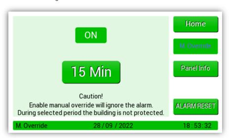
Pressing the ON/OFF button enables the override. There are four pre-set override time periods available. 15, 30, 45 and 60 minutes. Once a time period is selected the "M.Override" button will change to blue and a countdown begins and runs for the selected time period.
