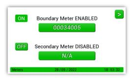
The example shows meter 1 enabled (on) and meter 2 off. If two pulse meters are being used both should be enabled here. To enable, or disable, a meter, press the on/off button on the screen.
