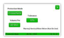
Crosscheck gives the panel flexibility to be used in applications where a comparison of two meters is required, e.g., a block of flats with heat interface units, especially useful if flats are left unoccupied for long periods. The flow and return into each flat can be monitored. If more water goes in than comes out, then the water loss will be noted by the panel resulting in an alarm condition.
