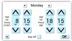
Set the start and end times required for high volume level. Any time outside of the time parameters here are considered low volume levels by the panel and will be measured as such, according to the volume levels selected in Protection Mode: Volume per. Tick 'Day Off' box to ignore that day.
