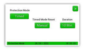
Timed does not measure volume. Instead, it will allow water flow for defined periods of time. (10, 15, 30 or 60 minutes). Any uninterrupted flow above this user defined time will put the system into alarm. In this example the unit is set for 10 minutes. If the water flows for 11 minutes the system will go into alarm. If the water runs for 9 minutes, stops, then flows for another 9 minutes, etc the system will not alarm.
