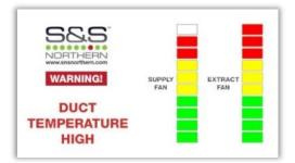
When the temperature drops below 30°C, system will automatically return to normal.
