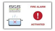
**FIRE ALARM ACTIVATED** If the connected fire panel detects a fire the gas and contactor will shut off. Fans can be driven in 4 combinations – *see settings.*
