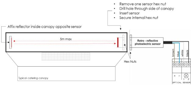
Sensor wired to Merlin 3000S circuit board
