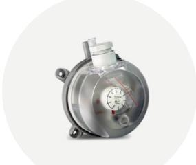
An air pressure differential switch is a mechanical switch fitted in ductwork which can be used to monitor and check airflow rates. These switches are adjustable and have a range from 20-300PA, they also come with a 1m duct kit to be fitted into the ductwork and detect the airflow.
