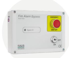
The Merlin FAB1 can be integrated with any of the Merlin suite of products to give the operator the opportunity to temporarily bypass the gas isolation system. With prior notice to a fire alarm test, the operator can turn the key to the on position giving an uninterrupted gas supply for between 10 and 45 minutes.
