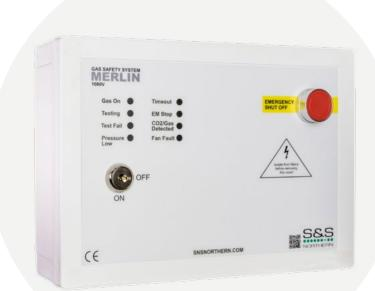
The Merlin 1000V+ gas pressure proving system is designed specifically for use in educational buildings and Laboratories with ventilation interlocking between the ventilation system and the gas solenoid valve. The system is compatible with external current monitors or air pressure differential switches in order to interlock with the ventilation units.
