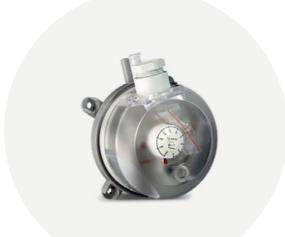
An air pressure differential switch is a mechanical switch fitted in ductwork which can be used to monitor and check airflow rates. These switches are adjustable and have a range from 20-300PA, they also come with a 1m duct kit to be fitted into the ductwork
