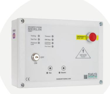
The Merlin 1000V+ gas pressure proving and electric isolation system is designed specifically for use in educational buildings and Laboratories with ventilation interlocking between the ventilation system and the gas solenoid valve. The system is compatible with external current monitors or air pressure differential switches in order to interlock with the ventilation units.
