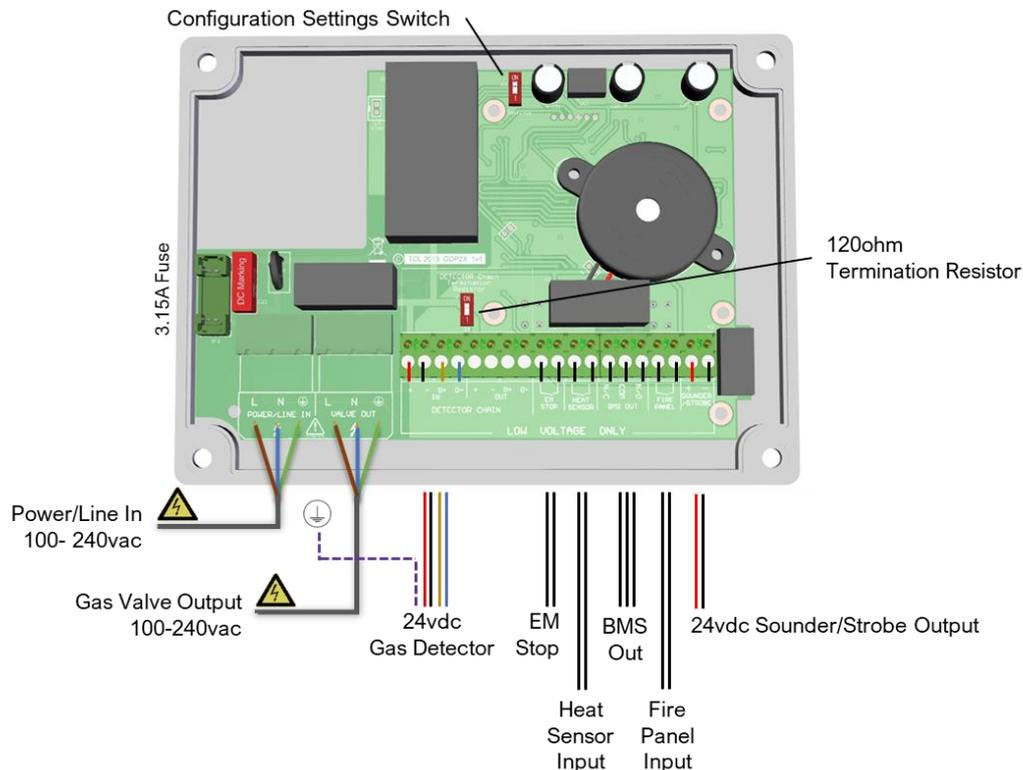
Note: Terminal blocks are plug/socket type and may be removed to ease wiring.
