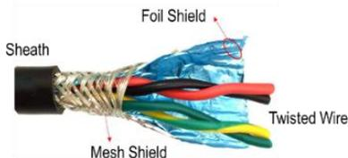
A shielded and twisted 2 or 4 core cable is used to wire the MODBUS terminals [D+ & D-]. The shielding can be of 2 types: braided [mesh of thin conducting wires] or foil (consisting of a thin sheet of metal covering the twisted wires). One example of such cable is BELDEN 3082A. Any cable with similar characteristics can be used to connect all the devices together.
