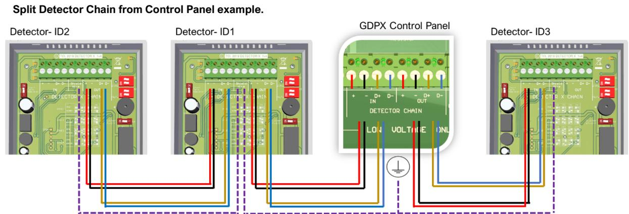
Reversing the [D+] and [D-] connections of any device can lead to the whole system to stop working owing to reverse polarity found on the terminals. In order to avoid this problem, it is recommended that a cable of same colour should be used to connect all [D+] terminals together and similarly cable of same colour to be used to connect all [D-] terminals together.
