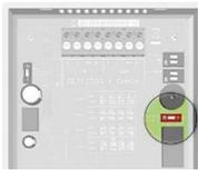
There is a switch on the detector board identified as [Buzzer On/Off]. The detector can be configured to have an audible alarm or not when gas levels reach the alarm set points. The alarm will continuously sound – there are no provisions to silence the alarm, gas levels must drop to a safe value for the alarm to stop.
