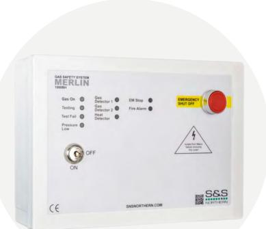
The Merlin 1000BH is a gas pressure proving and gas detection panel for use in plant rooms and boiler houses. This panel is to be used to carry out a gas proving test on the pipe work in order to highlight if there is a gas appliance open or a gas leak. The Merlin 1000BH is designed to give the user full control over the incoming gas supply with the lockable keyswitch operation.
