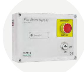
The Merlin FAB1 can be integrated with any of the Merlin suite of products to give the operator the opportunity to temporarily bypass the gas isolation system. With prior notice to a fire alarm test, the operator can turn the key to the on position giving an uninterrupted gas supply for between 10 and 45 minutes.
