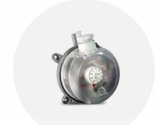
An air pressure differential switch is a mechanical switch fitted in ductwork which can be used to monitor and check airflow rates. These switches are adjustable and have a range from 20-300PA, they also come with a 1m duct kit to be fitted into the ductwork and detect the airflow.
