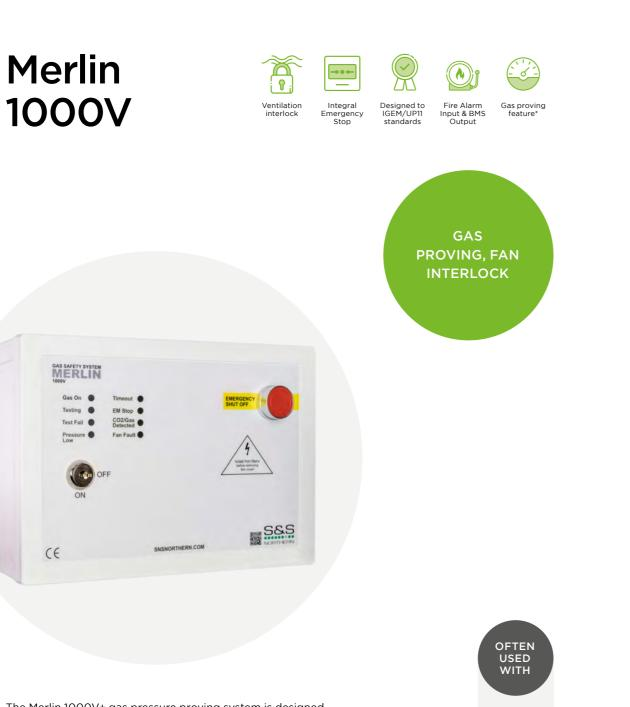
The Merlin 1000V+ gas pressure proving system is designed specifically for use in educational buildings and Laboratories with ventilation interlocking between the ventilation system and the gas solenoid valve. The system is compatible with external current monitors or air pressure differential switches in order to interlock with the ventilation units.
