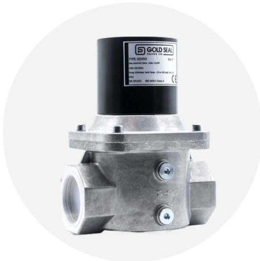
Our gas solenoid valves are 230V powered, normally closed, auto-reset and will most commonly be powered from our Merlin gas safety systems. In the event of an emergency, the Merlin gas safety system will take power away from the gas solenoid valve causing it to slam shut, and when power is re-instated this will then allow gas to flow through the pipework.
