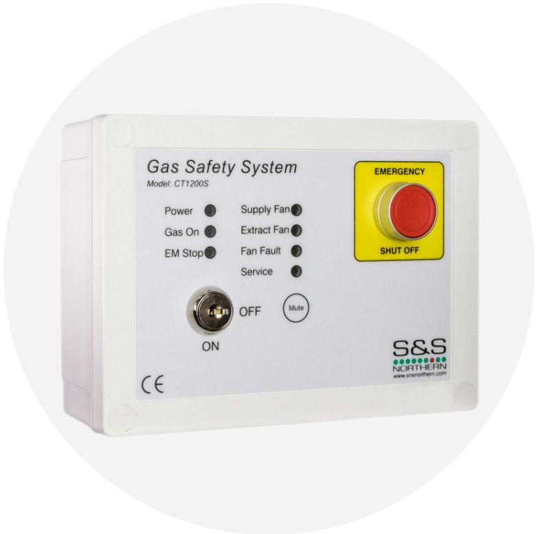
The Merlin CT1200S System is a gas interlock system for commercial kitchens. This can monitor ventilation using air pressure differential switches or external current switches.
