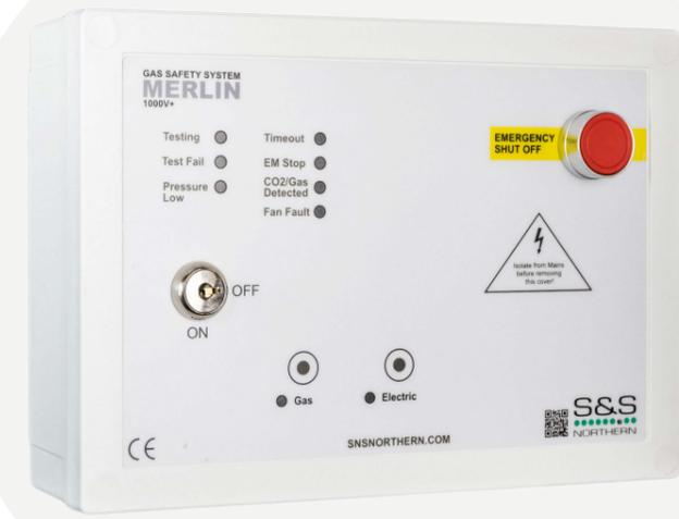
The Merlin 1000V+ gas pressure proving and electric isolation system is designed specifically for use in educational buildings and Laboratories with ventilation interlocking between the ventilation system and the gas solenoid valve. The system is compatible with external current monitors or air pressure differential switches in order to interlock with the ventilation units.
