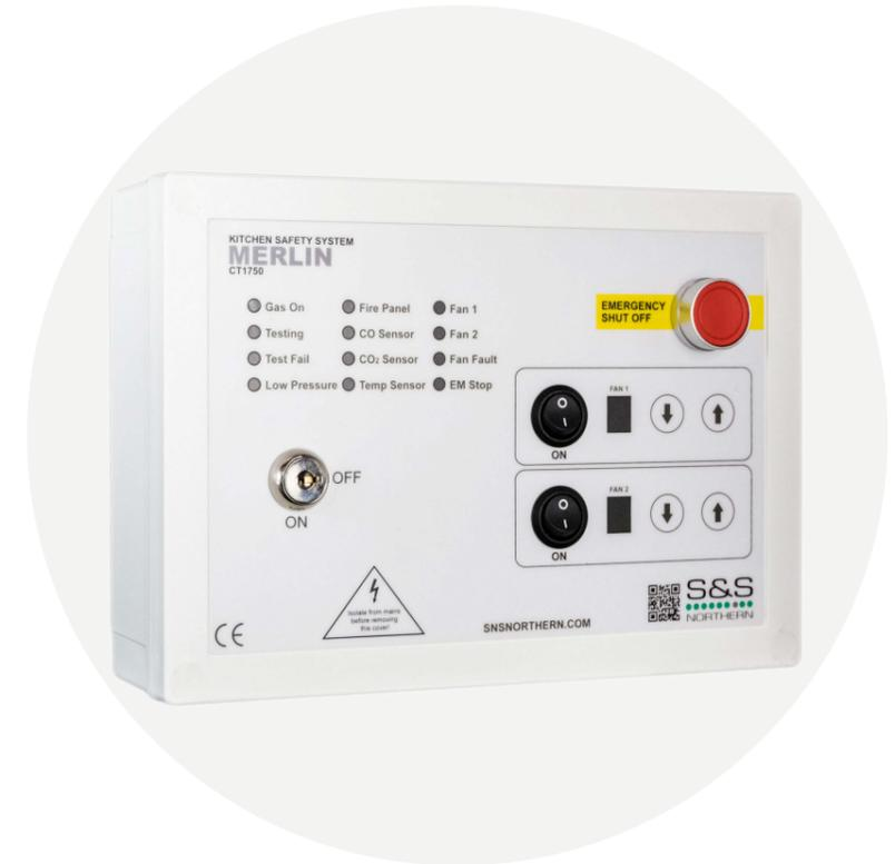
The Merlin CT1750 System is a gas interlock and manual ventilation control system designed for commercial kitchens. The Merlin CT1750 System comes with two variable fan speed controllers (0-10V output) to control the speed of 2 fans via an inverter.
