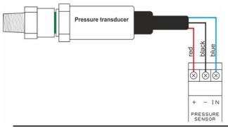
These wire to the gas pressure sensor which is screwed into the downstream port of the gas solenoid valve.
