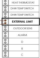
Typical Boiler Low Volt Control Board
