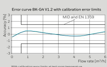
With calibration error limits at test room temperature Error curves of BK-G1.6 and BK-G4 are available on request
