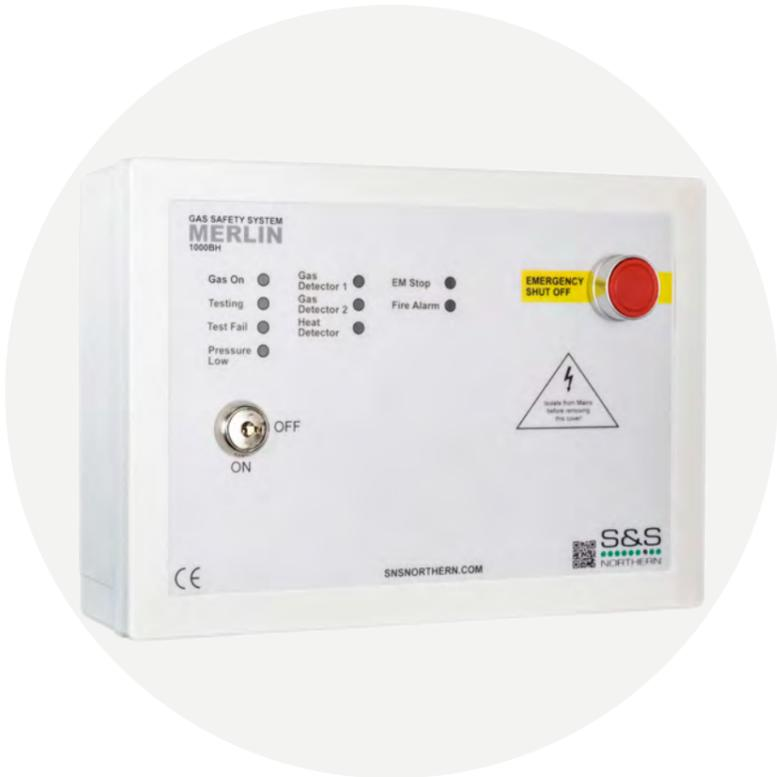
The Merlin 1000BH is a gas pressure proving and gas detection panel for use in plant rooms and boiler houses. This panel is to be used to carry out a gas proving test on the pipe work in order to highlight if there is a gas appliance open or a gas leak. The Merlin 1000BH is designed to give the user full control over the incoming gas supply with the lockable keyswitch operation.
