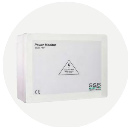
The Merlin PM2+ Current Monitor is a dual fan current monitor and is to be used in conjunction with the Merlin systems: the unit can be used as an alternative to an air pressure differential switch.
