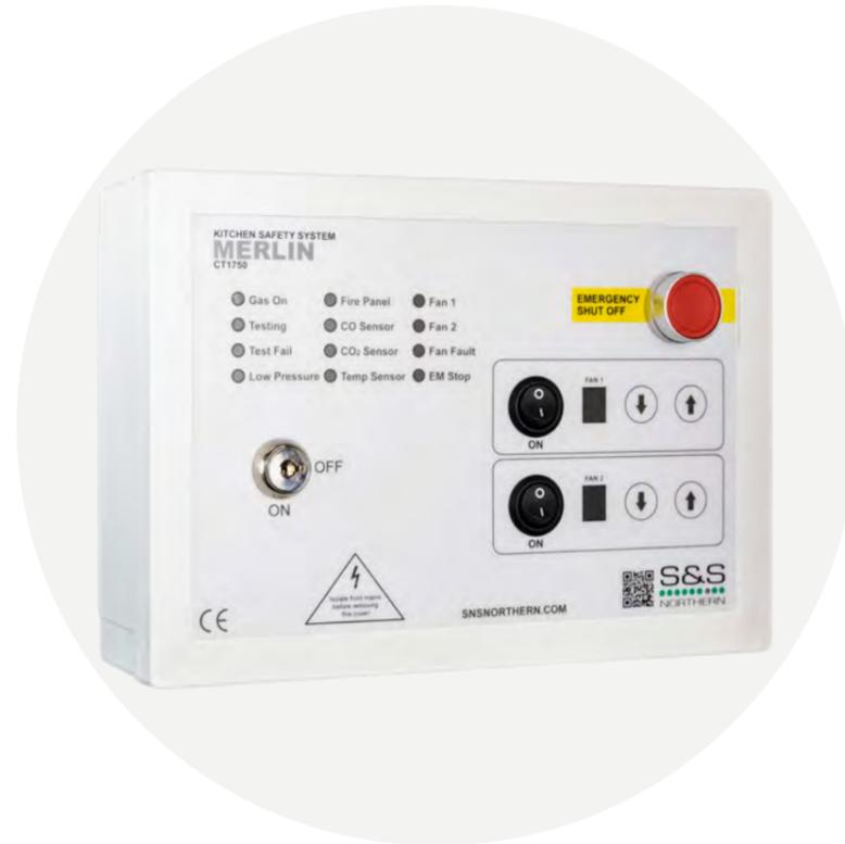
The Merlin CT1750 System is a gas interlock and manual ventilation control system designed for commercial kitchens. The Merlin CT1750 System comes with two variable fan speed controllers (0-10V output) to control the speed of 2 fans via an inverter.
