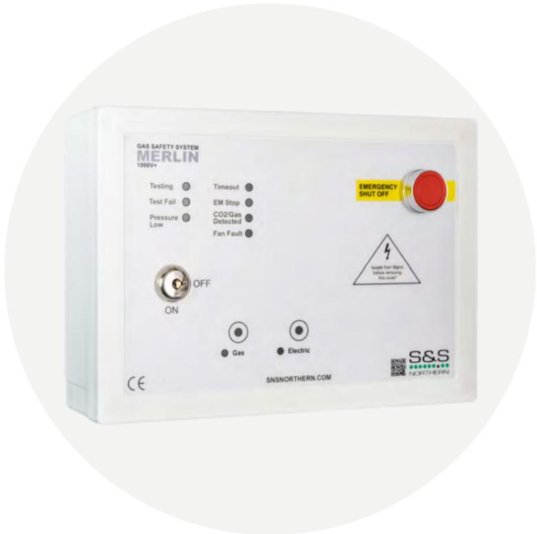
The Merlin 1000V+ gas pressure proving and electric isolation system is designed specifically for use in educational buildings and Laboratories with ventilation interlocking between the ventilation system and the gas solenoid valve. The system is compatible with external current monitors or air pressure differential switches in order to interlock with the ventilation units.
