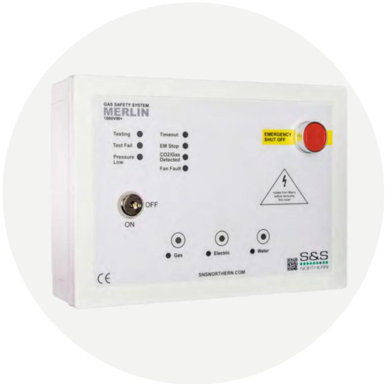
The Merlin 1000VW+ gas pressure proving, electric and water isolation system is designed specifically for use in educational buildings and Laboratories. The 1000VW+ can also interlock any mechanical ventilation.
