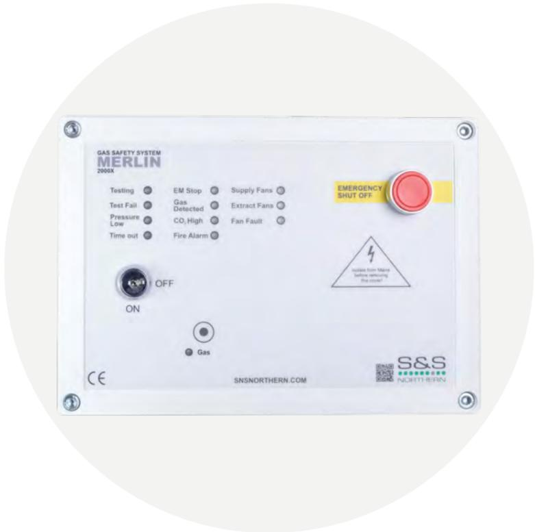
The Merlin 2000X is a ventilation interlock and gas proving system for commercial kitchens and includes two built in intelligent current monitors.
