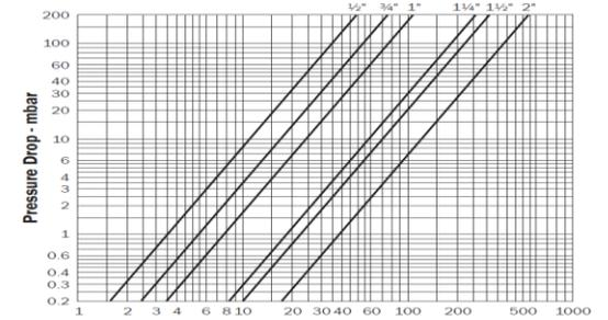
Based on +15°C, 1013 mbar, dry **Air Flow - Nm³/h**
