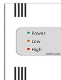
⚠ **High** - If the High LED flashes and buzzer beeps, there is a fault – contact your supplier.
