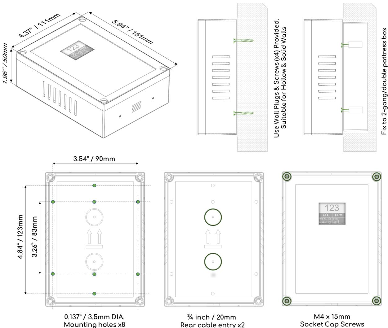
1. Carefully remove the front cover from the unit by using an M3 socket wrench.
