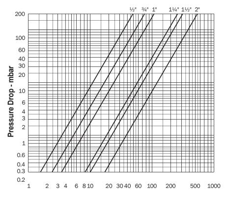
Based on +15°C, 1013 mbar, dray Air Flow - Nm<sup>3</sup>/h
