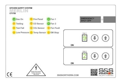
When the system is connected to the mains supply, the red LED of the S&S logo located in the bottom right corner of the panel will illuminate. When no power is present, this LED will not light.
