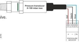
Connect the pressure sensor as shown: Wiring: Red [+] Black [-] Blue [IN]
