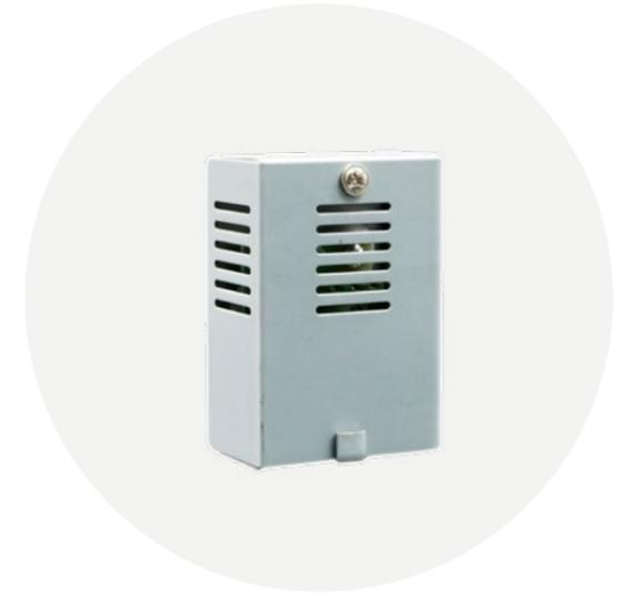
The fusible link is most commonly used in a boiler room application. These are fitted as a means of fire protection, if the boiler room temperature reaches over 72 degrees then the fusible wire inside will melt and therefore send an electronic signal to isolate the gas supply. Multiple fusible links can be fitted in one area.
