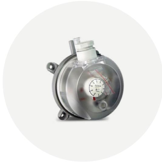
An air pressure differential switch is a mechanical switch fitted in ductwork which can be used to monitor and check airflow rates. These switches are adjustable and have a range from 20-300PA, they also come with a 1m duct kit to be fitted into the ductwork and detect the airflow.
