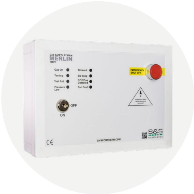
The Merlin 1000V+ gas pressure proving system is designed specifically for use in educational buildings and Laboratories with ventilation interlocking between the ventilation system and the gas solenoid valve. The system is compatible with external current monitors or air pressure differential switches in order to interlock with the ventilation units.
