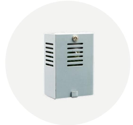
The fusible link is most commonly used in a boiler room application. These are fitted as a mean of fire protection. If the boiler room temperature reaches over 72 degrees then the fusible wire inside will melt and therefore send an electronic signal to isolate the gas supply. Multiple fusible links can be fitted in one area.
