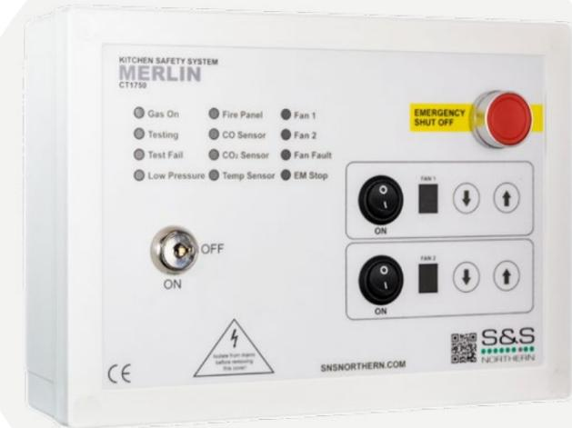
The Merlin CT1750 System is a gas interlock and manual ventilation control system designed for commercial kitchens. The Merlin CT1750 System comes with two variable fan speed controllers (0-10V output) to control the speed of 2 fans via an inverter.
