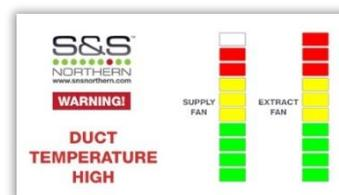
When the temperature in the extraction duct drops below 73°C, the warning screen will disappear and the fans will continue at a speed dependant on the temperature.
