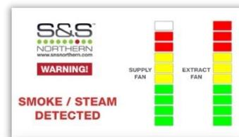
When smoke or steam is not detected continuously for ~5 seconds the system will automatically return to normal.
