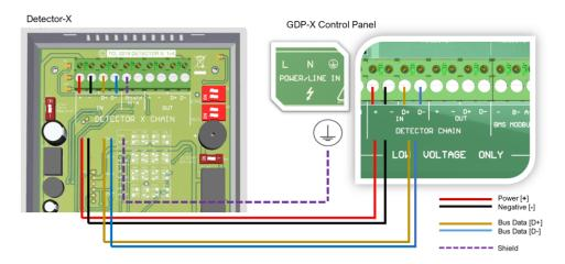
[SHEILD WIRE] detector terminals used for earthing/grounding and shield wires connected to any earth/ground terminal on the control panel. Twist the shield wire to avoid stray shield wires. If the detector does not have dedicated shield wire terminals, shield wires connect to the 24vdc negative terminal [-] on both detector and panel.
