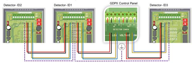
Reversing the [D+] and [D-] connections of any device can lead to the whole system to stop working owing to reverse polarity found on the terminals. In order to avoid this problem, it is recommended that a cable of same colour should be used to connect all [D+] terminals together and similarly cable of same colour to be used to connect all [D-] terminals together.
