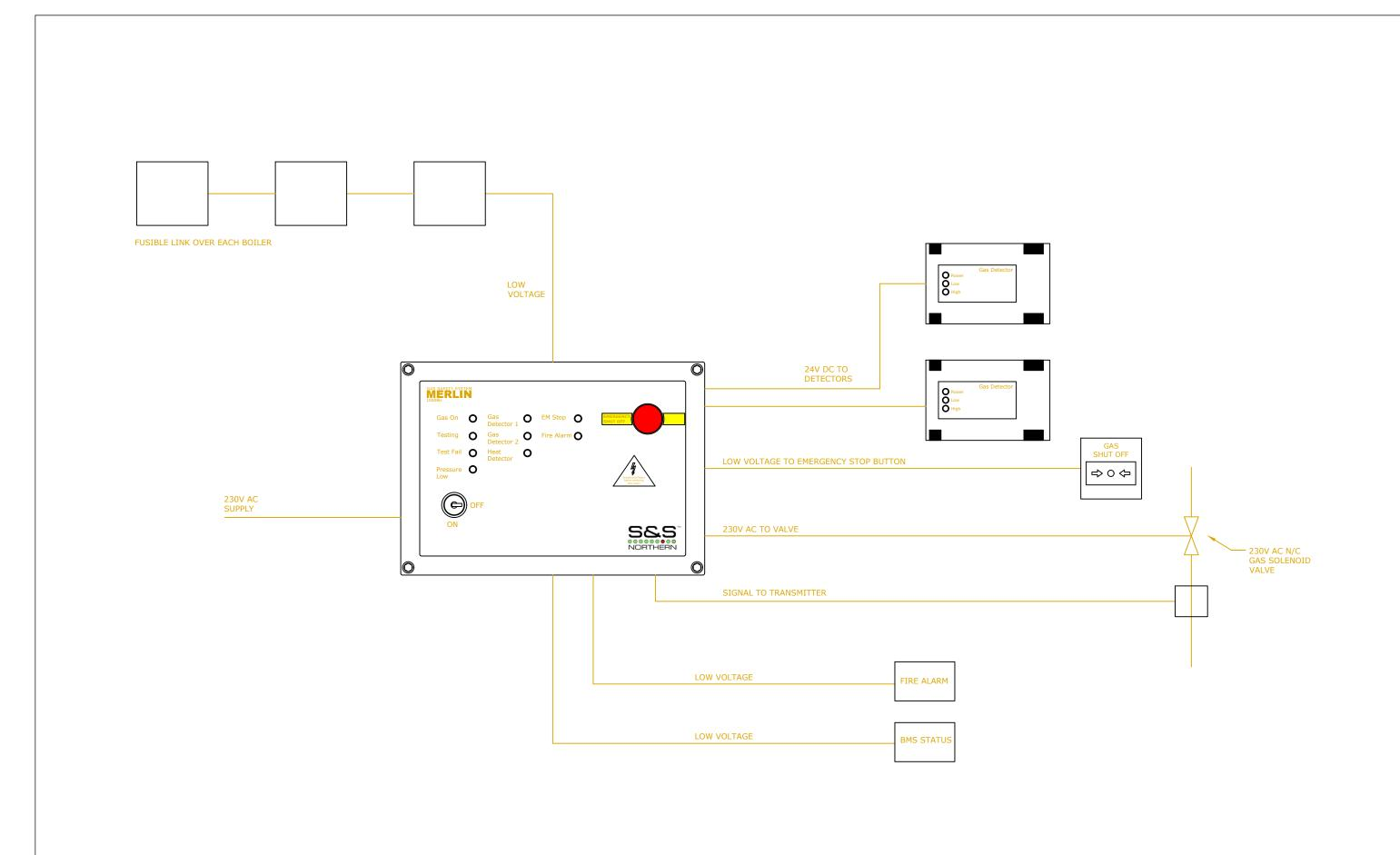
MERLIN 1000BH 2 ZONE GAS DETECTION & PRESSURE PROVING SYSTEM
