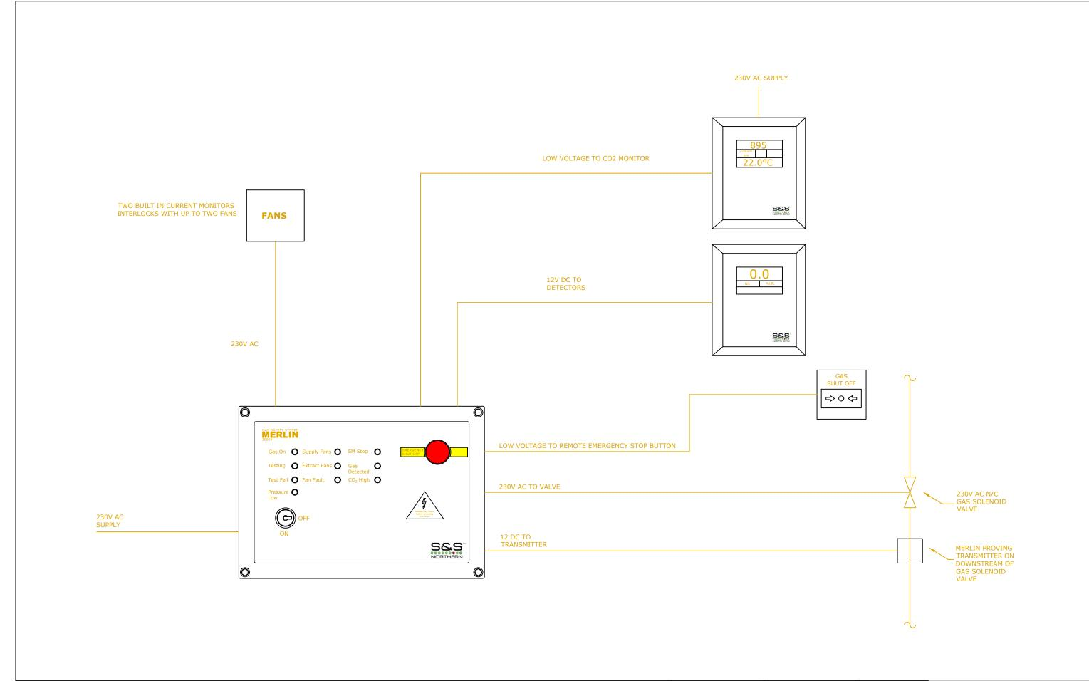
MERLIN 2000X GAS PROVING & VENTILATION INTERLOCKING SYSTEM WITH TWO BUILT IN ADVANCED CURRENT MONITORS
