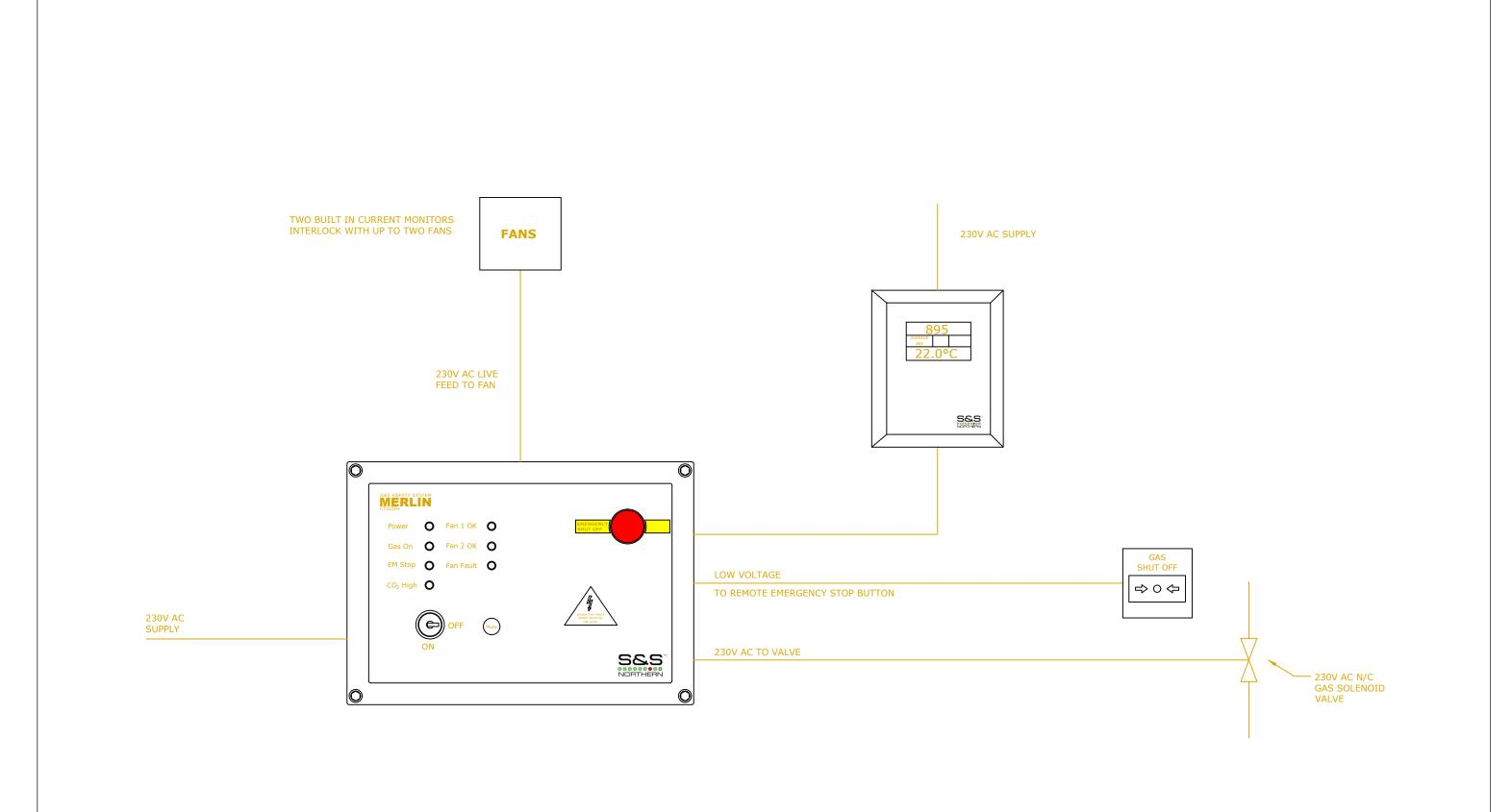
MERLIN CT1650+ GAS INTERLOCKING SYSTEM WITH TWO BUILT IN ADVANCED CURRENT MONITORS
