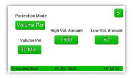
In this mode the system will allow a set amount (volume) of water through the pulse meter during a defined period. By combining these values, you increase/decrease the sensitivity of the systems measurement of flow volume. To edit the flow volume, press the button under the high or low volume value you wish to adjust. Use the arrows to adjust values, press enter to save and return to the screen shown.
