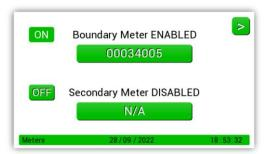
The example shows meter 1 enabled (on) and meter 2 off. If two pulse meters are being used both should be enabled here. To enable, or disable, a meter, press the on/off button on the screen.
