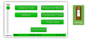
When the settings switch is turned on, the panel screen will display the settings menu. When setup is complete, turning off the switch will save all settings.
