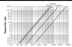
Based on +15°C, 1013 mbar, dry Air Flow - Nm3/h
