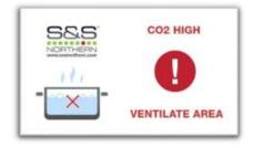
**CO<sub>2</sub> HIGH** When CO<sub>2</sub> gases rise above alarm level (see CO<sub>2</sub> Monitor manual) the fault screen will appear. The gas and contactor will shut off and fans will run at maximum speed.
