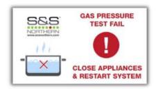
**GAS PRESSURE TEST FAIL** If the gas pressure test drops by more than 10% below 12mBar the test will fail.
