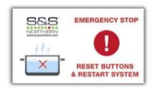
**EMERGENCY STOP** If an emergency stop button (remotely or direct) is pressed, the gas and contactor will shut off. Fans can be driven in a combination upon emergency stop activation— *see settings*. The Emergency Stop must be reset before restarting the system.
