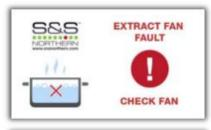
**SUPPLY & EXTRACT FAN FAULT** If a supply or extract fan fault is detected for longer than 20 seconds - the gas, contactor and fans will all shut off.
