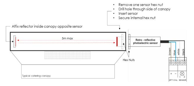
Sensor wired to Merlin 3000S circuit board
