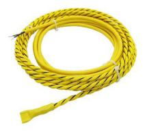
WLMC 2-Core leak detection ropes include a 2M lead wire, however this wire may be extended using alarm cable. The total length of lead wire and sensing cable may not exceed 60M. If more than 60M is required, use multiple WLM controllers.
