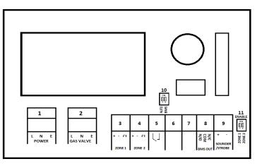
Note: Terminal blocks are plug/socket type and may be removed to ease wiring.
