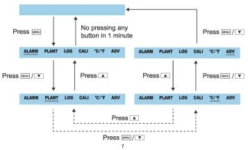
To select the function, press when it is underlined by the flashing bar. Note that after 1 minute if nothing is pressed, the Main Menu will disappear and the device will revert to the normal state.
