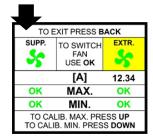
If calibration is unsuccessful then alter fan dropout thresholds in the settings menu and repeat.
