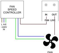
The live feed from the fan controller should be connected to either the supply or extract side depending on which fan/s are being monitored.
