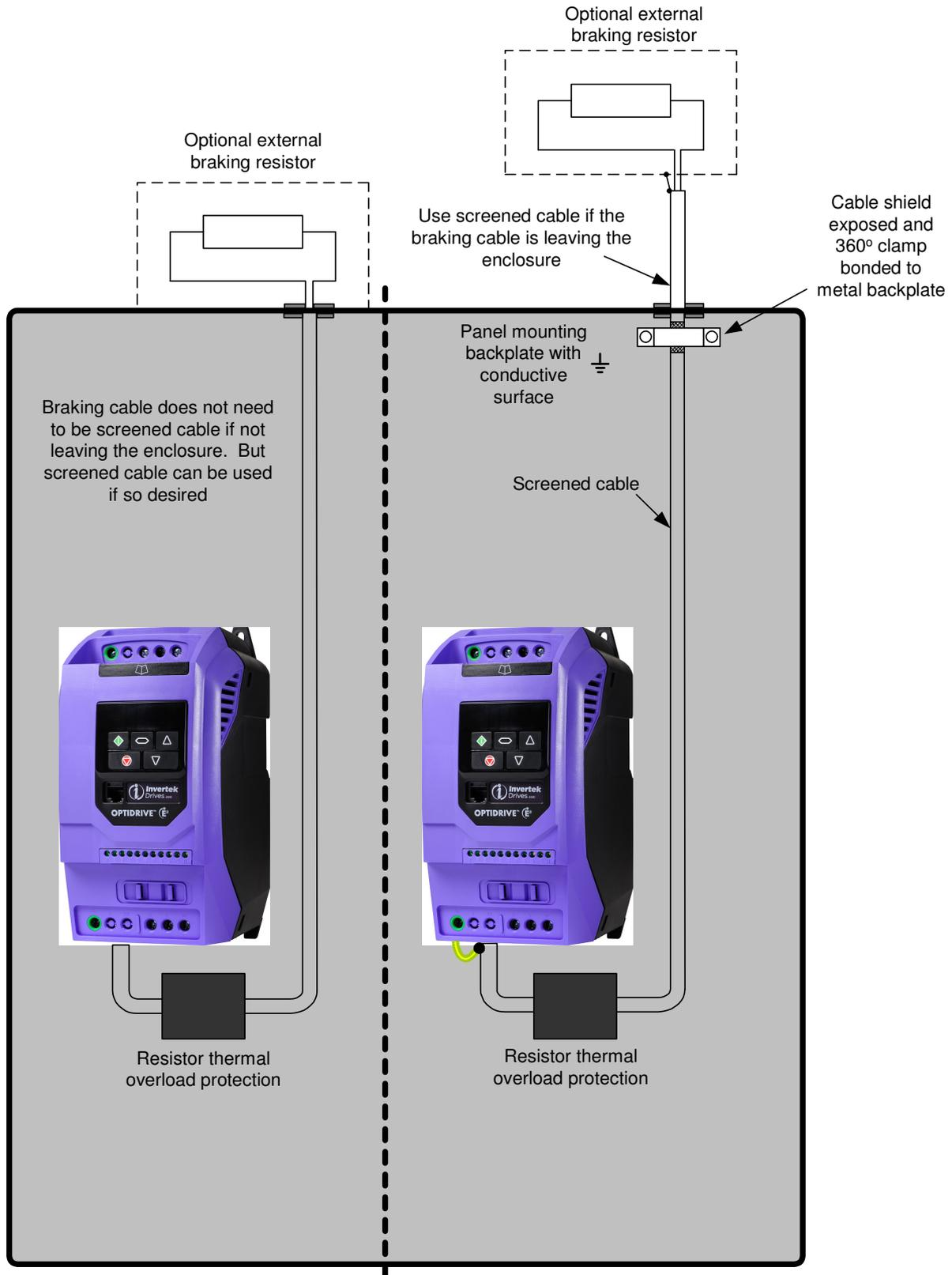
**Note:** Some earth cables have been omitted for clarity. Please make sure braking resistor and case are properly earthed.
