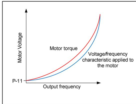
**NOTE:** If parameter P-13 is set to 1 or 2 (pump or fan mode), setting parameter P-06 (Energy optimizer) to a 1 will have no effect. If P-06 = 2 or 3, the Optidrive E3 energy optimization is enabled.
