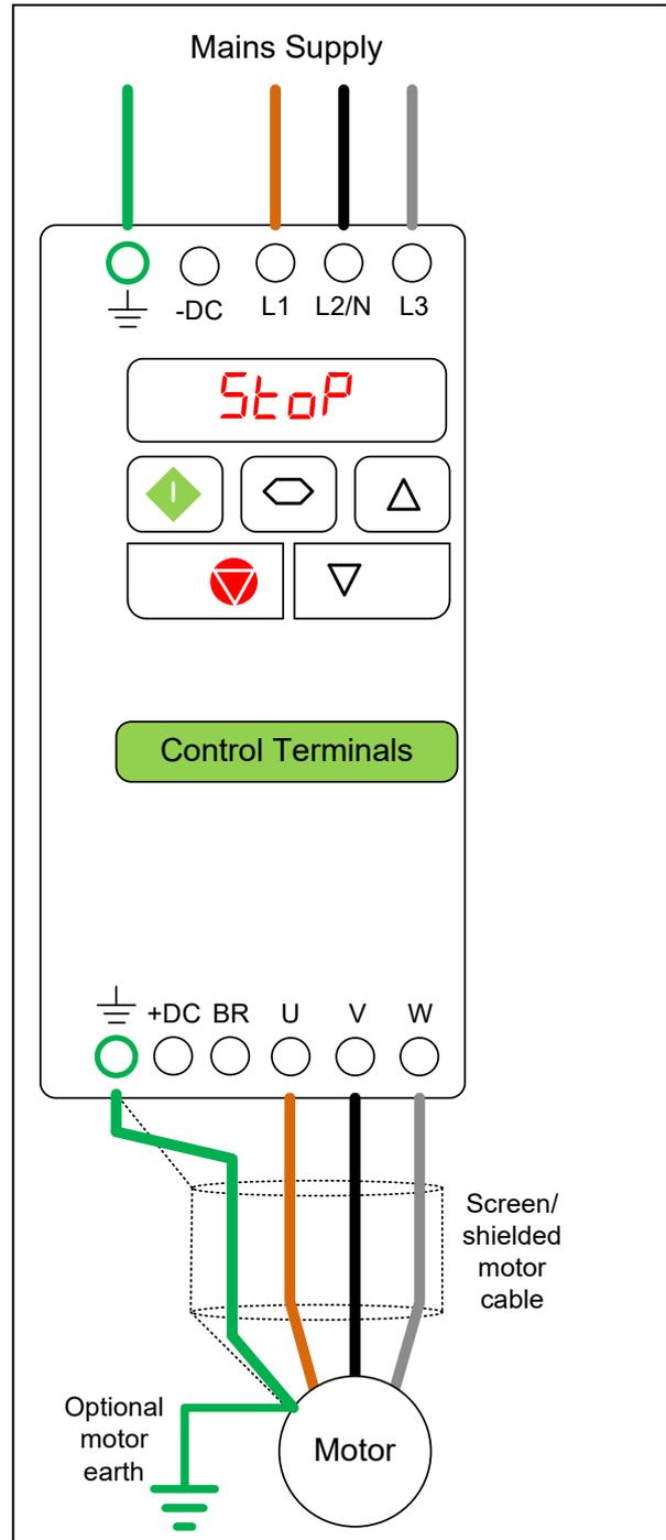
**NOTE:** On E3 size 4 & 5, there are earth connections on the drives heatsink at the top and bottom of the drive
