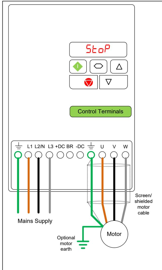
**NOTE:** For information on connecting a braking resistor, see Section 15 – Dynamic Braking
