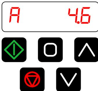
Press and release the NAVIGATE button, the display will show Output power:
