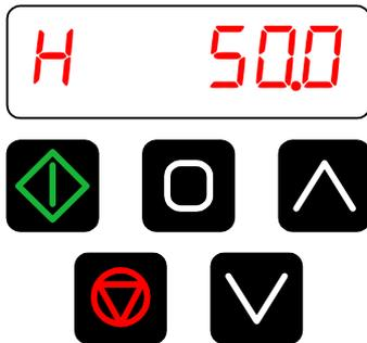
Press and release the NAVIGATE button, the display will show Output current:
