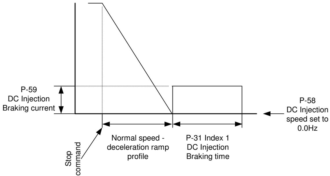
**DC Injection Braking On Stop (Inject DC at 50Hz)**
