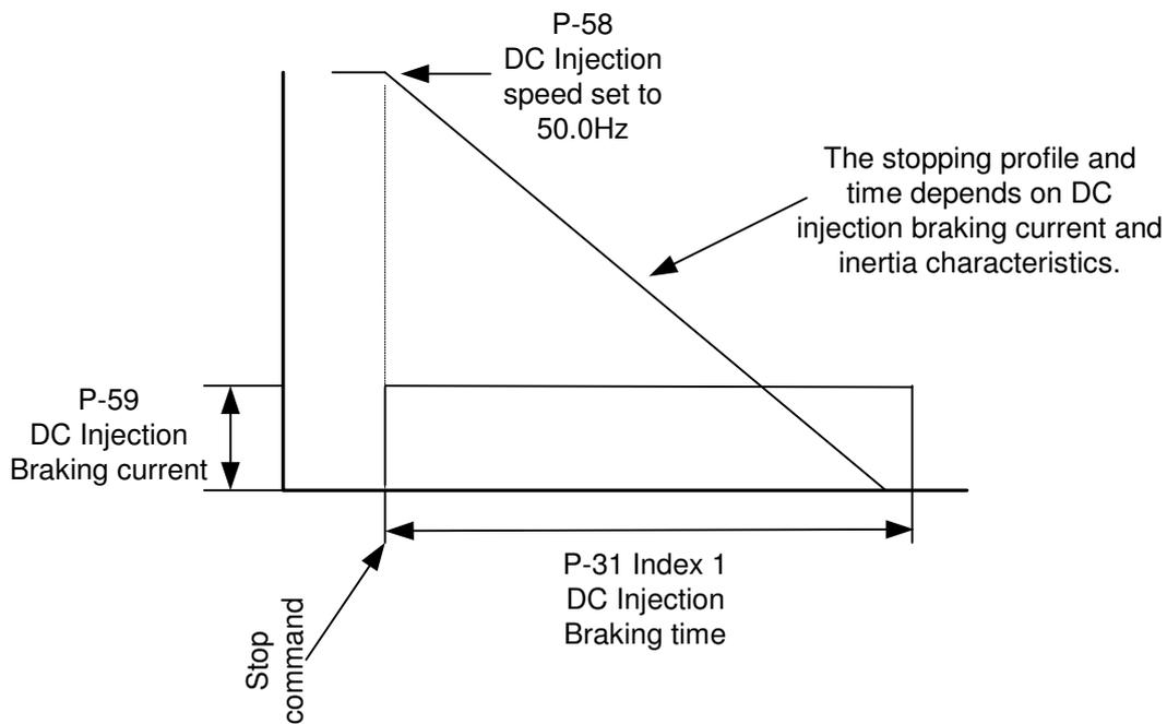
DC Injection Braking On Stop (Inject DC at 30Hz)
