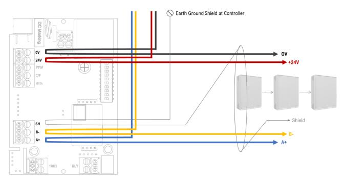
Daisy chain wires running to additional RS sensors – 127 sensors max per cable run. First and last device in bus requires a termination resistor. Use EOL switch to terminate RS sensor. Recommended 3-core, 2 twisted pair + ground, shielded cable with 120  $\Omega$  characteristic impedance.
