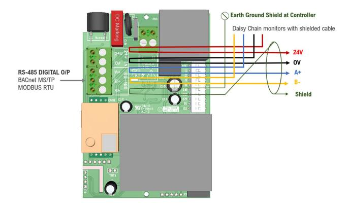
Daisy chain wires running to additional monitors – 127 sensors max per cable run. First and last device in bus requires a termination resistor. Use EOL switch to terminate IAQ sensor. Recommended 3-core, 2 twisted pair + ground, shielded cable with 120  $\Omega$  characteristic impedance.
